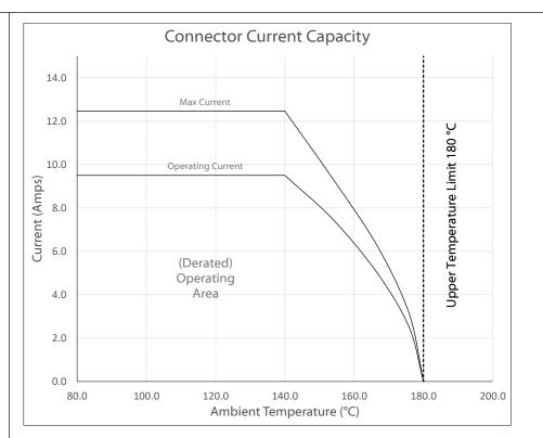
Testing based on IEC 60512-5-2. Max current curve generated with isolated test article under controlled environmental conditions, based on a 40°C temperature rise difference. Test does not take into account external factors such as housings,mating cables, or other circuitry. Operating current curve (derated by 20% of maximum values) accounts for external factors, and manufacturing variation.
