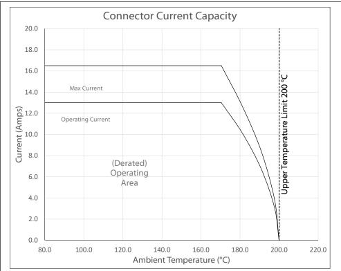
Testing based on IEC 60512-5-2. Max current curve generated with isolated test article under controlled environmental conditions, based on a 40°C temperature rise difference. Test does not take into account external factors such as housings, mating cables, or other circuitry. Operating current curve (derated by 20% of maximum values) accounts for external factors, and manufacturing variation.
